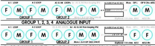
Gp 1& 2 ANALOGUE IP, Gp 3 & 4 AES (with DEMODULATED OP on the D-25)
